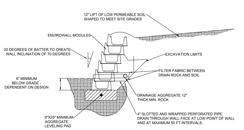
IMPORTANT: GRAVITY WALL LIMITED TO NO MORE THAN 6 TOTAL BLOCK COURSES TALL AT ANY LOCATION ON THE WALL. TALLER GRAVITY WALLS ARE POSSIBLE WITH SITE SPECIFIC DESIGN PREPARED BY AN EXPERIENCED PROFESSIONAL ENGINEER.
