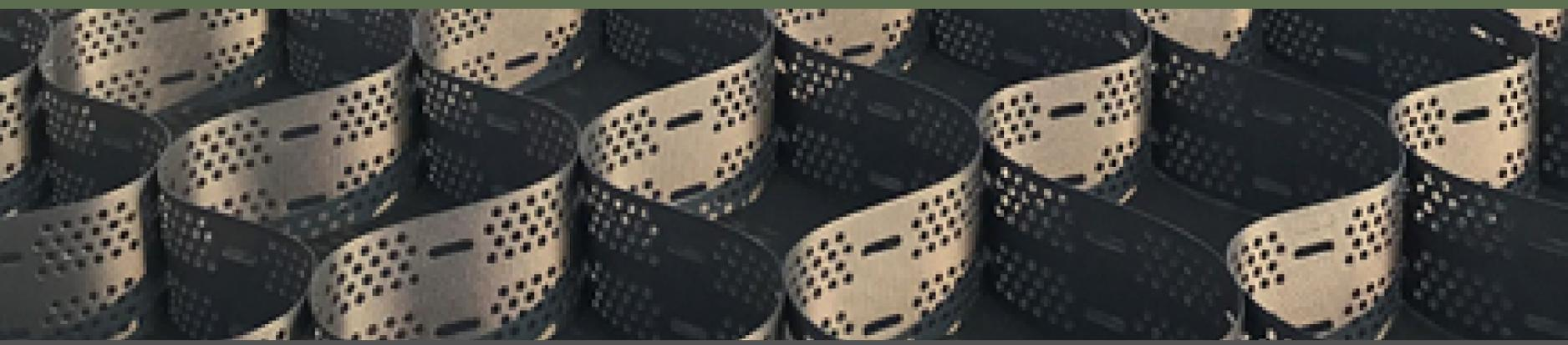
When first pulled open, the cells will have the tendency to open in an hourglass shape. When proper length is reached, pull the panel edges to insure rectangular expansion. Then, stake the panels at each cell along the width at either end, and along the cell every other cell. Straight re-bar or wooden stakes can be used.
