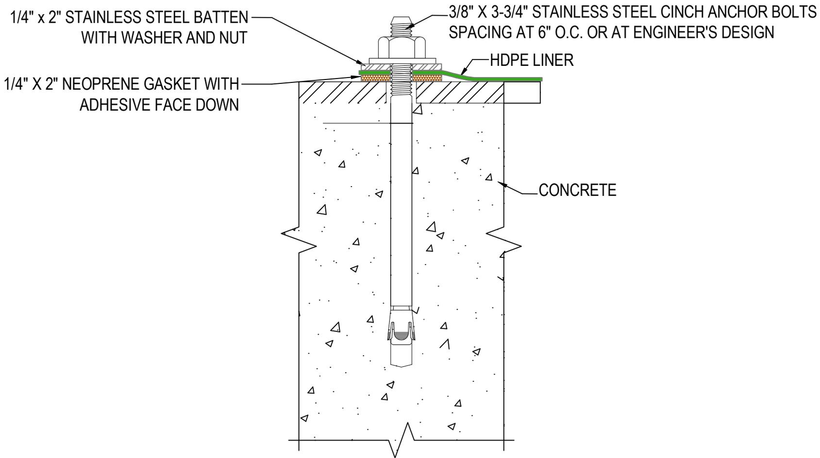
**TYPICAL CONCRETE ANCHOR - PROFILE VIEW**
